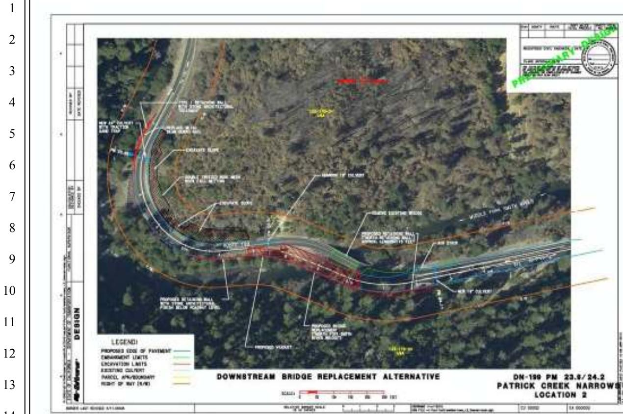
15        100. The work here would involve excavation of 20,000 CY from the slopes above
