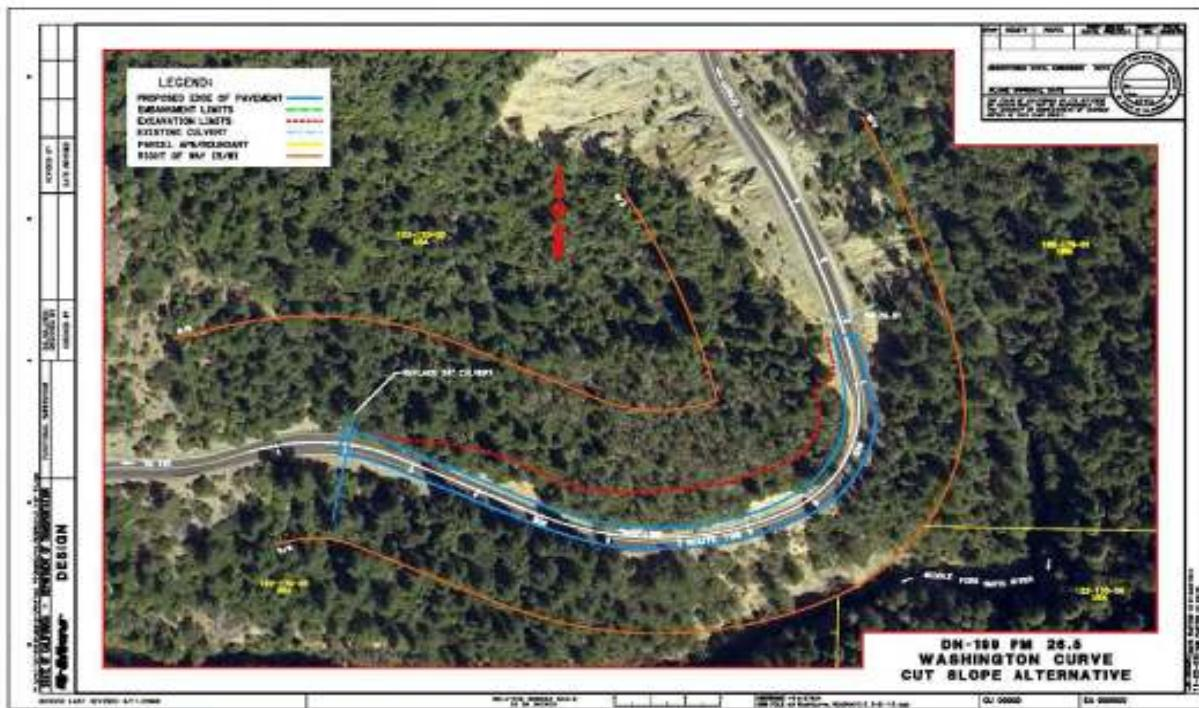
119. The excavation calls for removal of approximated at 23,00 CY of soil, with the
